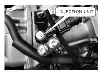
3. OIL PUMP: Sucking the fuel into the pump from the fuel tank and injecting it into the oil pipe by high pressure. (If the oil can't get into the engine or the acceleration is not good, you need to check the pump)
